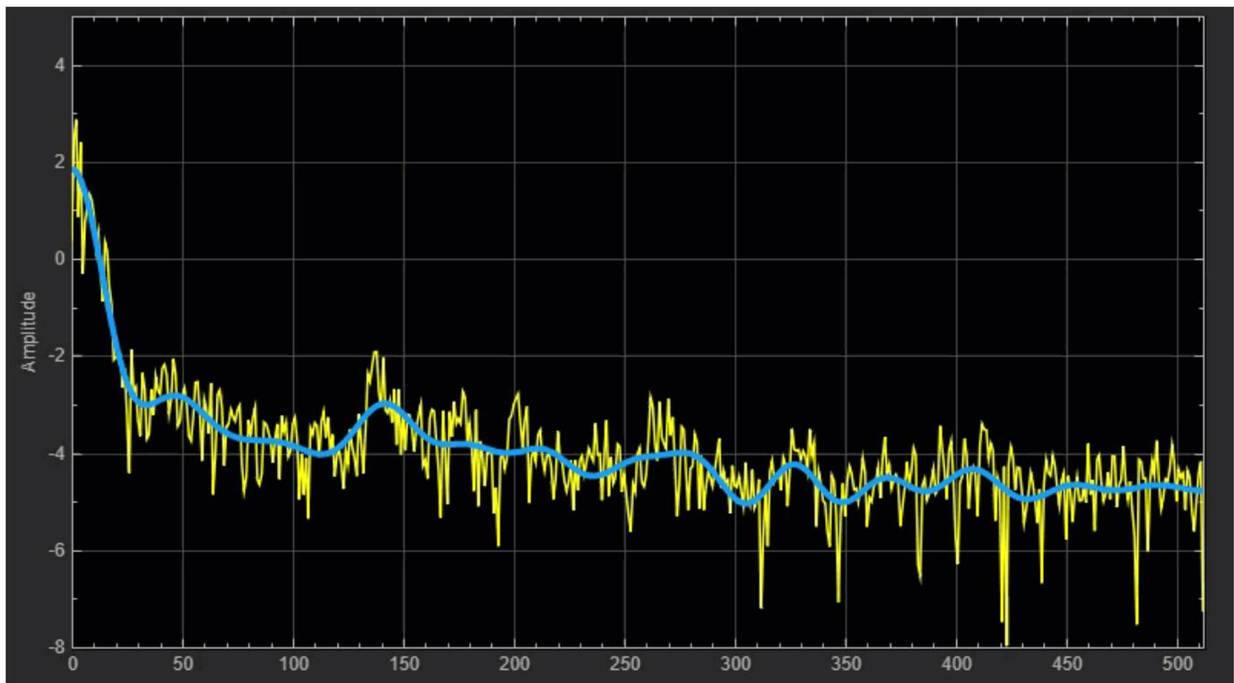
The loop ends if either a maximum number of iterations (`100`) is reached, or if all bins of the estimated log envelope are within a given tolerance of the original log spectrum. The tolerance is set to  $\log(10^{(1/20)})$ .
